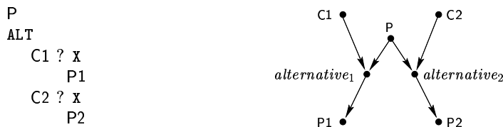
Figure 1: A dynamic precedence graph representing P : the output mode of P is ALT and the input mode of alternative_1 and alternative_2 is PAR .
