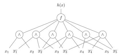
Figure 1: A depth-2 circuit  $h:\{0,1\}^5 \to \{0,1\}$  where the top gate is a function  $f:\{0,1\}^6 \to \{0,1\}$  and the bottom level gates are AND gates on a subset of the input bits and their negations. More generally, we consider  $h:\{0,1\}^n \to \{0,1\}$ , with top gate  $f:\{0,1\}^m \to \{0,1\}$ .
