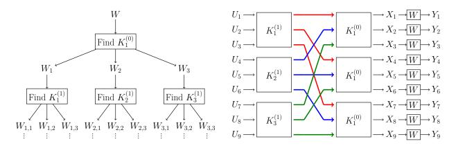
Figure 1: The left figure illustrates the code construction, and the right figure shows the encoding procedure for the special case of  $\ell = 3$  and t = 2. All the kernels in this figure have size  $3 \times 3$ . One can show that the bit-channel  $W_{i,j}$  in the left figure is exactly the channel mapping from  $U_{3(i-1)+j}$  to  $(U_{[1:3(i-1)+j-1]}, Y_{[1:9]})$  in the right figure.
