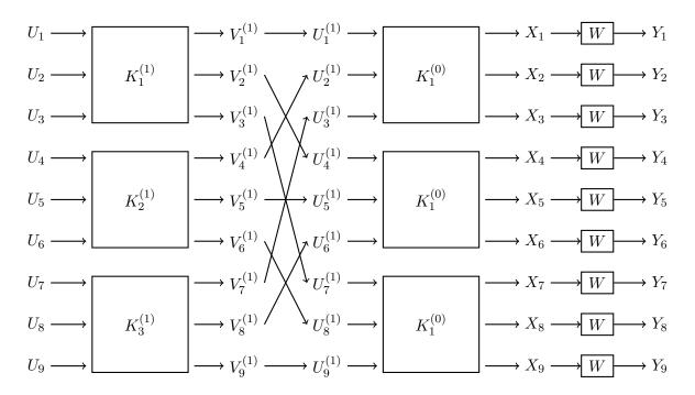
Figure 3: Illustration of the encoding process  $\mathbf{X}_{[1:N]} = \mathbf{U}_{[1:N]} M^{(t)}$  for the special case of  $\ell = 3$  and t = 2. Here  $\mathbf{X}_{[1:N]}$  and  $\mathbf{U}_{[1:N]}$  are row vectors. All four kernels in this figure  $K_1^{(0)}, K_1^{(1)}, K_2^{(1)}, K_3^{(1)}$  have size  $3 \times 3$ , and the outputs of each kernel is obtained by multiplying the inputs with the kernel, e.g.  $\mathbf{V}_{[1:3]}^{(1)} = \mathbf{U}_{[1:3]} K_1^{(1)}$ .
